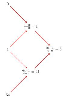
Thus  $f[x_0, x_1] = 1$ ,  $f[x_0, x_1, x_2] = 5$  and the Newton form of the quadratic interpolating  $f(x) = x^3$  at 0, 1 and 4 is given by
